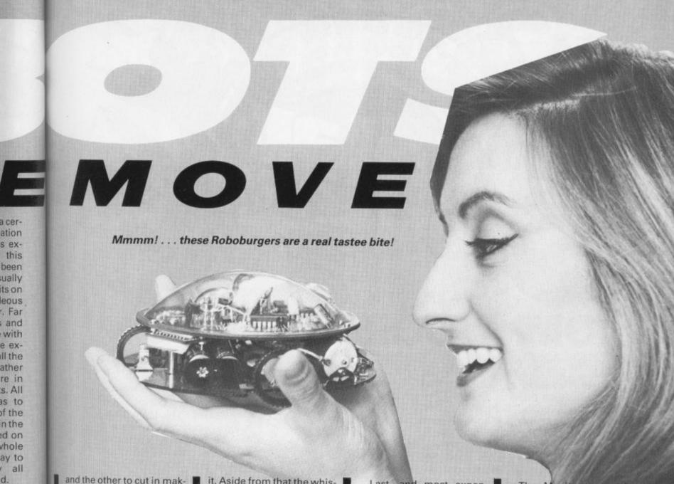
and the other to cut in making it change direction. If the corners are tighter than its turning circle (about 20 cms) it wanders off and does its own thing against the nearest wall. The kitchen floor nearly gave it a nervous breakdown. The sensor underneath is very sensitive, even picking up pencil marks on paper and it responds very quickly even on lines a good deal thinner than those recommended for use.
